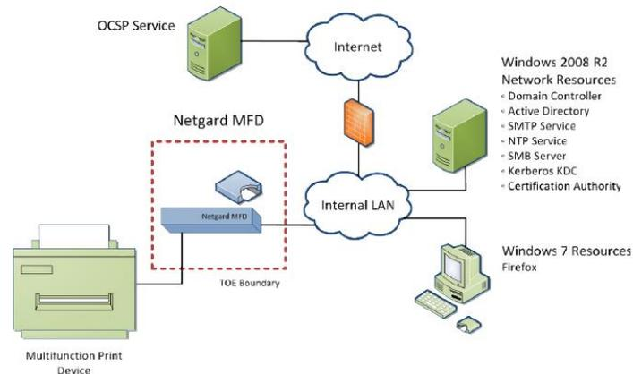
**Figure 1 TOE Architecture**
